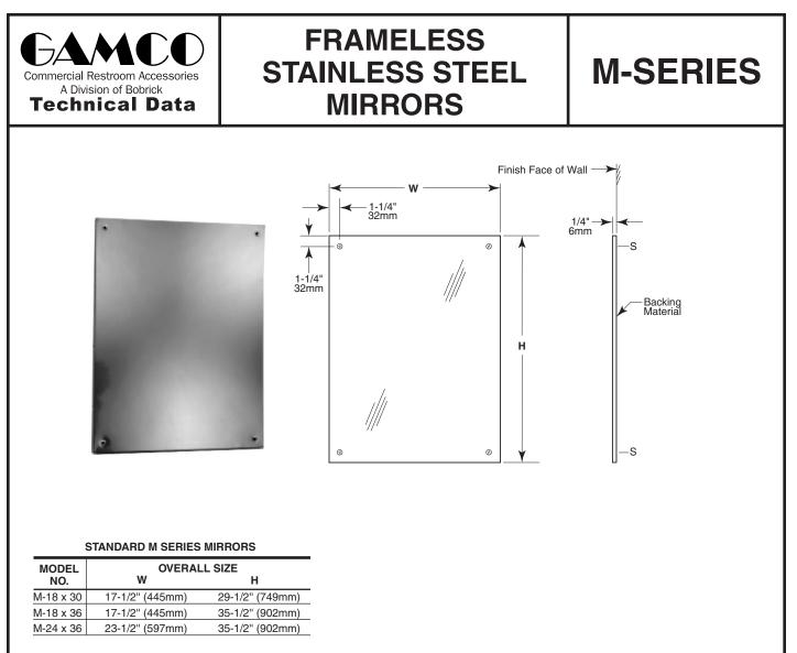
Note: Overall width and height of custom M-Series mirrors will be 1/2" (12mm) smaller than dimension specified.
