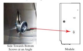
On cabinets deeper than 4", using provided template, new holes can be made on the module closer to the front door to make it easier to install the module and will allow the lower screw heads to sit flush against the cabinet surface.
